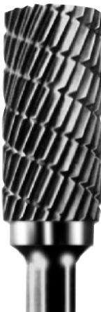
Standard cut with chipbreaker. Used for tempered, unhardened steel, cast steel and weld seams.
